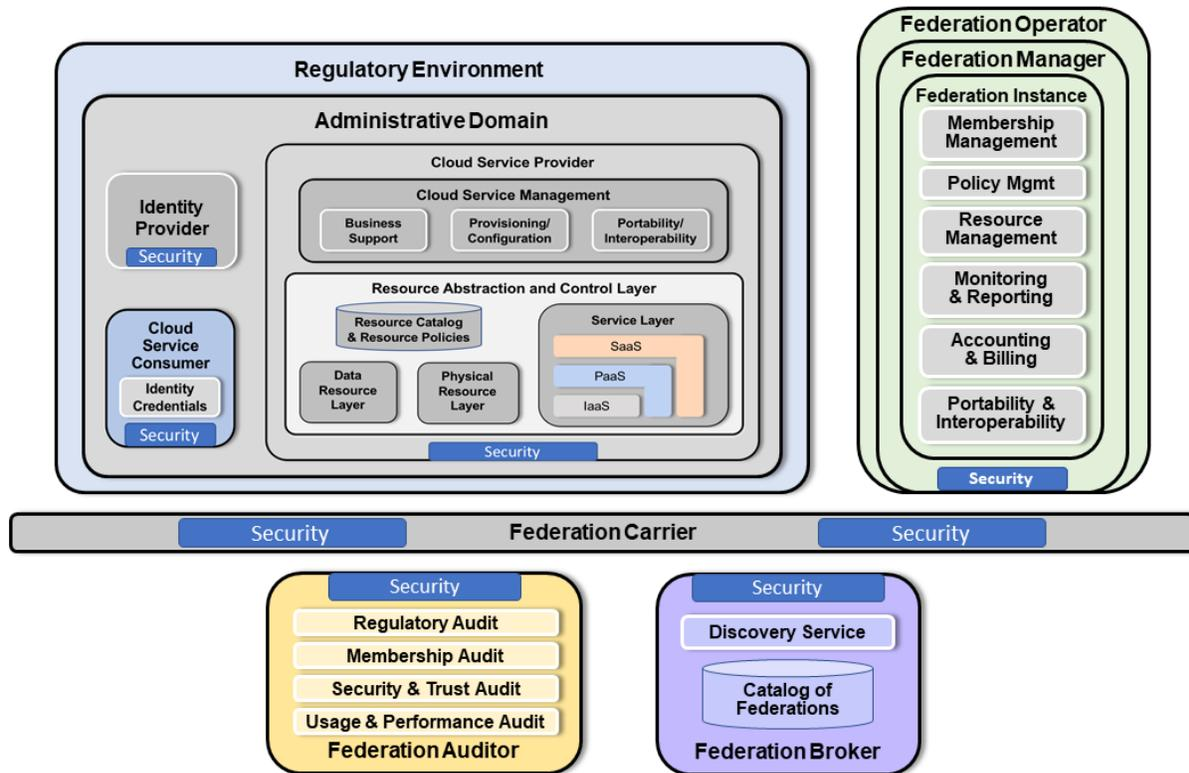
**Figure 4.** The NIST Cloud Federation Reference Architecture Actors.
